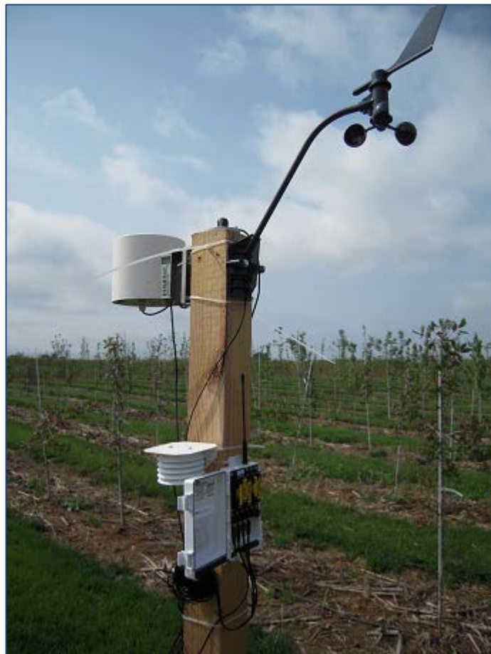
Figure 13. It is recommended that you install a weather station node at your operation. It is invaluable for providing information about your microclimate, and is used by the software to calculate a number of factors (degree days, chill hours, etc.).
